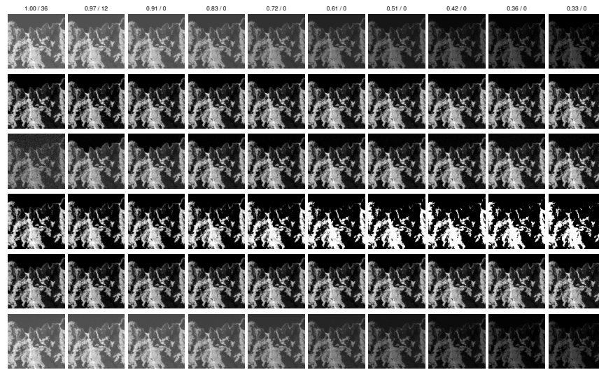
Fig. 3. Abundance maps of the first endmember used in the synthetic mixtures (theoretical abundances on the first line, VCA/FCLS on the second line, SISAL/FCLS on the third line, \ell_{1/2} NMF on the fourth line, BCD/ADMM on the fifth line, proposed method on the last line). The top line indicates the theoretical maximum abundance value and the true number of pixels whose abundance is greater than 0.95 for each time instant.
