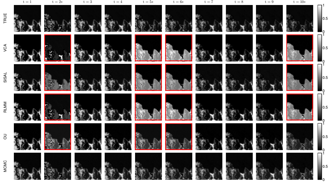
Fig. 4. Abundance map of the first endmember recovered by the different methods (in each row) at each time instant (given in column) for the experiment with R = 3 [the different rows correspond to the true abundances, VCA/FCLS, SISAL/FCLS, RLMM, OU and the proposed method]. The images delineated in red show that several methods are highly sensitive to the presence of outliers, and the time instants represented with * denote images containing outliers.
