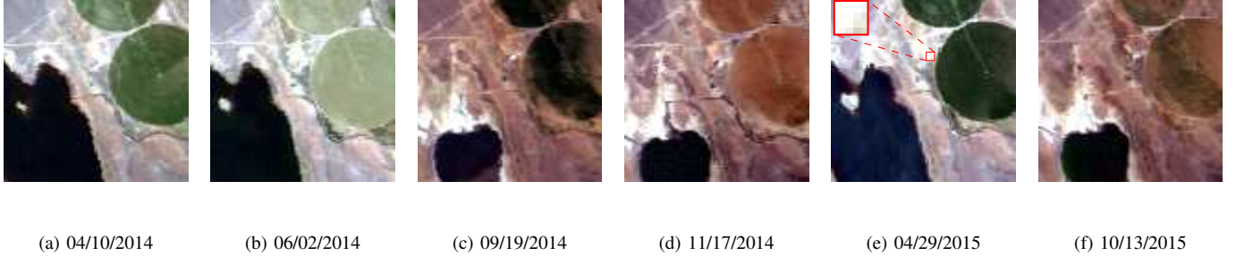
Fig. 5. Mud lake dataset used in the MTHS experiment with the corresponding acquisition dates. The area delineated in red in Fig. 5(e) highlights a region known to contain outliers (this observation results from a previous analysis led on this dataset in [31]).
